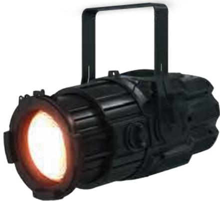
Tenore 3 and 5 boast a Fresnel lens offering a wide zoom range of 12° to 68°, give or take depending on their LED source. These fixtures can be available with PC lens instead, with a tighter beam starting from 7°. Optional 4- or 8-leaves barndoors are available on request.
