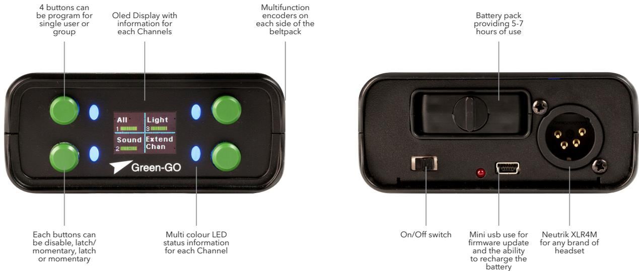
The WPBX Wireless Beltpack uses DECT wireless technology to communicate with the WAA antenna, providing the same features and flexibility that you're already familiar with from the Green-GO wired system. This allows for users to seamlessly switch from wired to wireless without having to learn a new system. Each WPBX Wireless Beltpack can be paired with up to four WAA antennas to extend the range as required.
