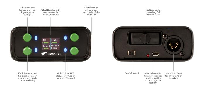
The WBPX Wireless Beltpack uses DECT wireless technology to communicate with the WAA antenna, providing the same features and flexibility that you're already familiar with from the Green-GO wired system. This allows for users to seamlessly switch from wired to wireless without having to learn a new system. Each WBPX Wireless Beltpack can be paired with up to four WAA antennas to extend the range as required.
