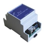
The node1 mkll is a surface mountable DMX / network node with DMX (input or output via 5-pin XLR) and network connection (Ethercon). Power is also supplied via the unit's Ethernet connection via PoE (Power over Ethernet). Programming is completed via the free ELC dmXLAN software.
