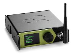
Aurora is the flexible unit able to transmit or receive one universe of DMX/RDM with several connectivity options. Using the intuitive color screen to change settings on the fly and move between universes, it is powerful enough for single universe transmissions as well as being a receiver packing the most advanced features.
