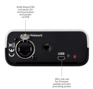
The BEACON signal light comes in the standard beltpack format and serves as an optical indicator for incoming communications, either a call, or a warning/go cue indication. In addition, the BEACON signal light can also be used as a blue luminous passing light.
