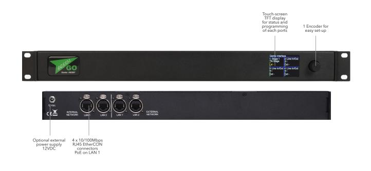
The Dante interface links up to 8 audio streams from and into the Green-GO network. The Dante interface will directly convert digital audio streams from Dante or AES67 to Green-GO and vice-versa, without the conversion losses that occur during analog to digital (and contrary) conversion.
